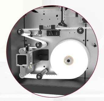
Main material label roll is unwinded passing through the guidance system to ensure accurancy during the process.
