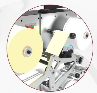
Lamination system add a self-adhesive material to the labeled main material.
